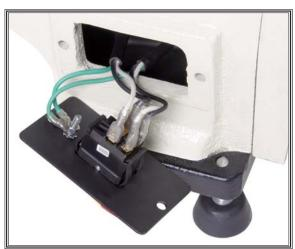
Figure 28. Switch connections.
